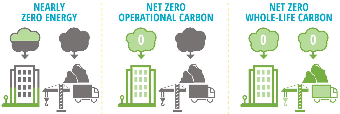
Figure 3: The difference in scope of the different building standards. Note the shift from energy (marked in yellow) to carbon (green) between the existing 'nearly zero energy' and the proposed net zero carbon standards.
